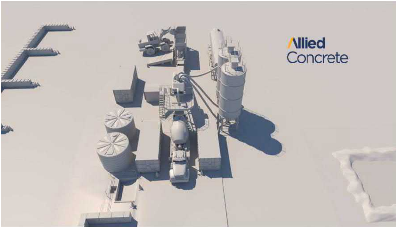
Figure 1: Two bin plant set up. Note: project will require two plants.
