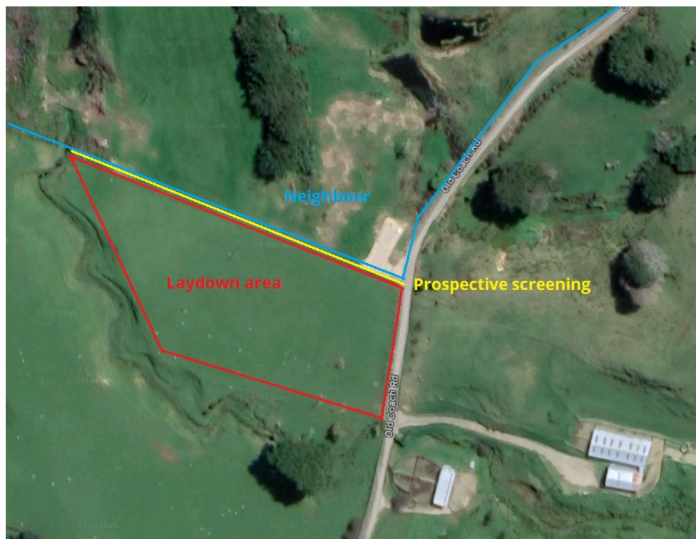
Figure 1: Property boundary screening location between the construction laydown area and the adjoining neighbour to the north
